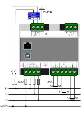
Figure 5: An example of a typical connection of SMC 233 in a LV network - wiring a measured voltage to a star in a four-wire network.
