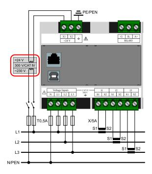
Figure 4: In a 300V/CAT IV network it is necessary to use a power supply with the corresponding overvoltage category! Our PWR1 or PWR3 smart grid power supply is conforming to this requirement.
