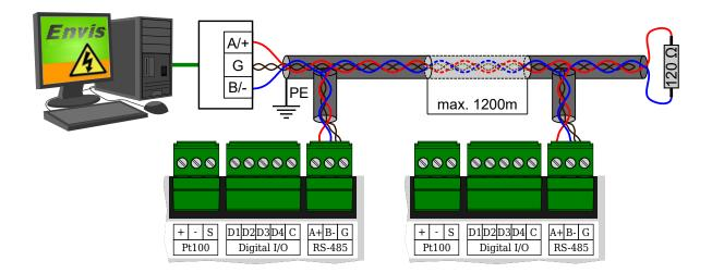
Figure 7: Connection of RS-485 communication lines to SMC 233 devices SMC 233.
