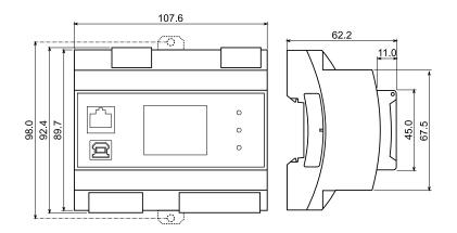
Figure 3: Dimensions of SMC 233.
