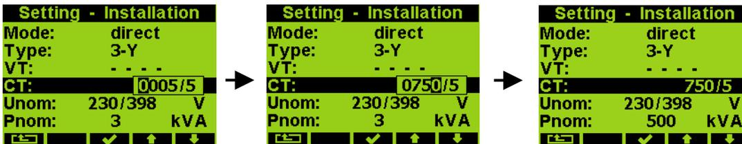
Now you can type new value of the parameter : with the **▶** button you can move from a digit to another one and to set each digit to target value using the **▲** and **▼** buttons. At the end press the **✓** button and the parameter is set.
