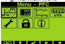
By pressing the **MENU** button, a *Main menu* window appears. With the **▶** and **◀** buttons you can browse through the menu and select a desired action with the **✓** button or return back using the **⏪** (escape) button.
