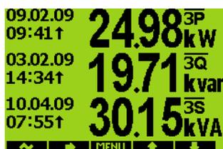
The maximums&minimums are displayed on the left side of average values window - maximum value is identified with the ↑ symbol and minimum value with the ↓ symbol.
