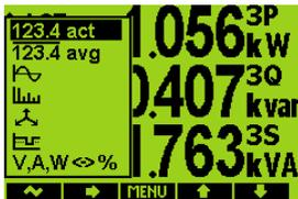
The actual data group comprises other actual data presentations that are accessible with the button - so called *actual data display mode switch* . When pressed, a pull up menu rolls over the display temporary. By multiple pressing of the button a desired actual data subgroup can be selected and displayed :
