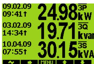
The maximums&minimums are displayed on the left side of average values window - maximum value is identified with the  $\uparrow$  symbol and minimum value with the  $\downarrow$  symbol.
