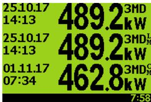
Only three-phase maximums with their time stamps are displayed. In the first row there is total maximum demand **3MD**, i.e. maximum of the 3AD reached since last maximum clearing. You can check this clearing time with the ► button – by **Clear** option selection, the clearing confirmation window appears and last maximum power demand clear time and current averaging parameters setting can be checked. If you don't want to clear the registered maximums, push the \*button, otherwise the ✓ button.
