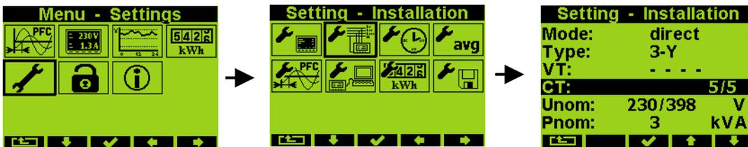
In the window navigate down to the current transformer ratio parameter ( CT ) and choose with the **✓** button.
