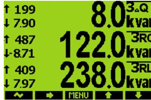
For compensation reactive power capacity assessment, registered minimum values of both reserves are decisive. On example on Fig. 4.20, registered minimum of three-phase capacitive reserve is 31.3 kvars, minimum of inductive reserve is 7.97 kvars. As both of them are positive the system compensation power is sufficient.
