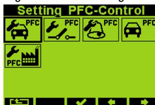
The complete PFC setting consists of a series of parameters arranged into three groups : **the PFC Control**, **the PFC Outputs** and **the PFC Alarms**. Next two options in the menu are **the Control <-> Manual** state toggle and **the PFC Factory Setting** utility.
