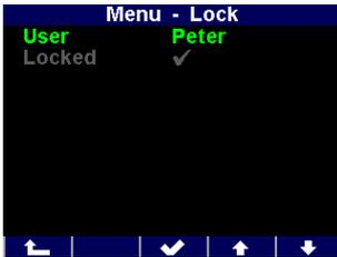
With the user management you can use more complex and sophisticated access control to the instrument not only from the instrument panel, but from all of communication interfaces.
