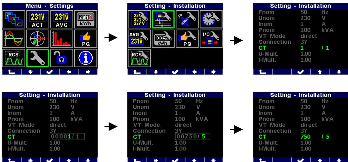
Now you can type new value of the parameter : with the you can move from a digit to another one and to set each digit to target value using the and . At the end press the and the parameter is set.
