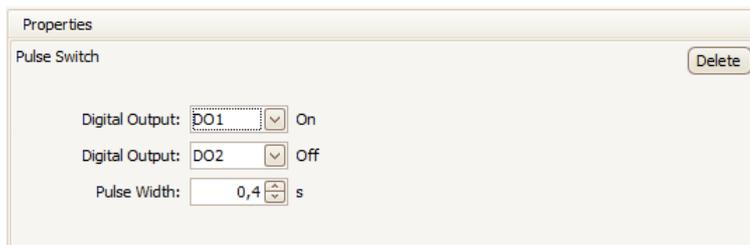
After the setup, if any change of the condition occurs, pulse of specified duration appears :
