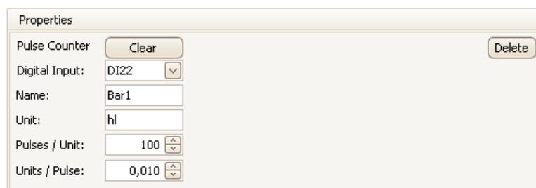
If the name is not defined, the quantity is referenced with its general name *PCxx* (when the *xx* is index corresponding digital input).
