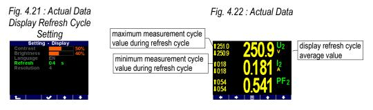
Actual values, read from an instrument via a communication link for monitoring purposes are evaluated from one – the last – measurement cycle only.
