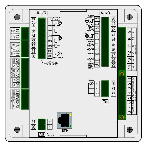
Inputs & outputs are connected to terminals on a rear panel of an instrument according to the following table.
