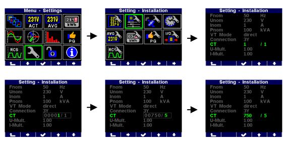
Now you can type new value of the parameter : with the vou can move from a digit to another one and to set each digit to target value using the rest and rest. At the end press the rest and the parameter is set.
