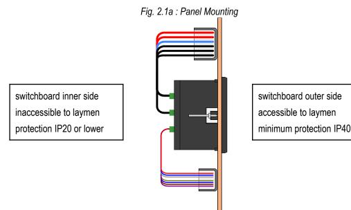
The instrument's position must be fixed with locks.
