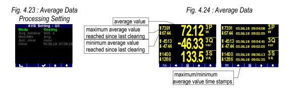
The maximum and minimum registered values can be cleared either manually or automatic clearing can be set.
