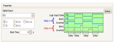
Fig. 6.20 : I/O Setup – Digital Input Condition Properties
