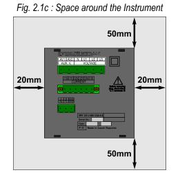
Especially underneath the instrument, no other instrumentation that is source of heat should be installed or the temperature value measured may be false.
