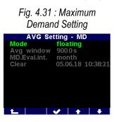
Parameters determining maximum demand processing can be set in the **Setting – AVG – MD** screen. As default, *the floating window* averaging method is set.
