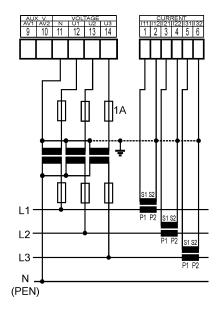
IT Network Delta ("3D") Connection via VT (VT to Line-to-Neutral Primary Voltage)
