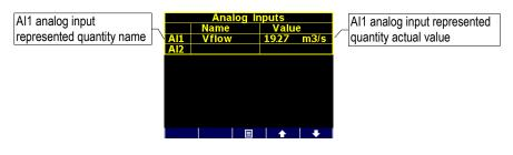
The analog input represented quantity value corresponds to actual input current or voltage at appropriate analog input according to the set ratio. At the example, the represented quantity *Vflow* has actual value of  $19.27 m^3/s$ .
